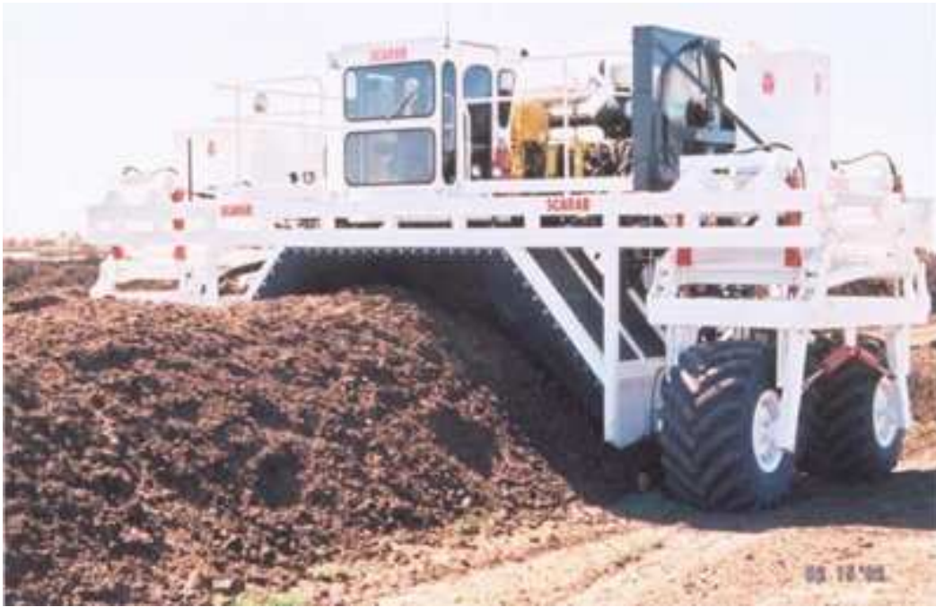
Picture of a SCARAB -- windrow turning equipment.
